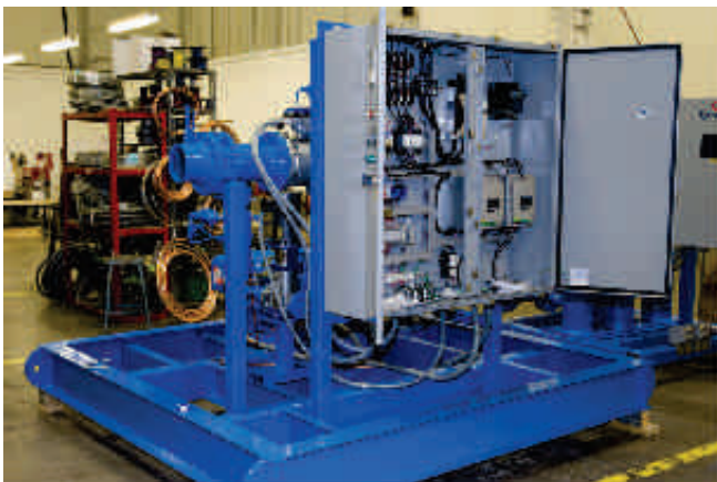
Skid mounted VFD panel
